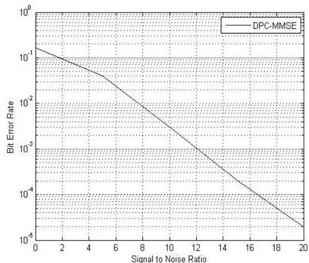
Fig.9 the BER (bit error rate) performance DPC pre-coding with MMSE equalizer
