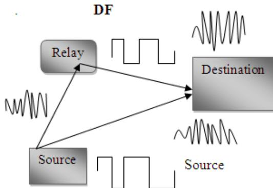
Fig.6 Decode and forward protocol
