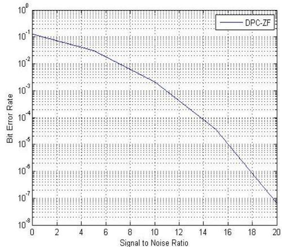
Fig.8 the BER performance of using ZF-DPC pre-coder
