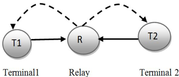
Fig.3 Two way relay network
